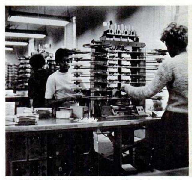
TWO DUBBINGS EMPLOYEES operate one of the firm's new duplicators. The machine enables the operators to duplicate 12 tapes from one master, or a total of 400 eight-track tapes per hour.
