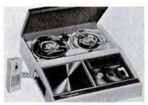
MAYFAIR PUSH-BUTTON. five-transistor tape recorder by Artic Import Co. Two micro motors, three-inch speaker, VU meter, fast forward control, speed control. Reel capacity 31/4 inch. Complete with remote control mike, two C batteries, earphone, tape and take-up reel. No price.
