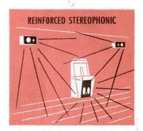
Position "C" directs the separate stereo channels to the stereo extension speakers and also combines both channels through the main unit speakers. In extra large or odd shaped locations where other equipment would require a "scatter-shot" speaker arrangement, Rock-Ola's four powerful 12" bass speakers and three high compression driver horns fully compensate for the location's acoustic deficiencies to provide smooth aural-balanced reinforced stereo sound.
