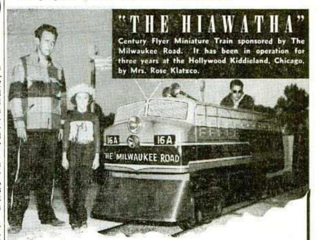
Do not confuse the Century Flyer with the narrow-gauge toy-type trains on the market today. It is a large train, operating on full 24 inch gauge track, capable of handling 140 passengers to the trip.
