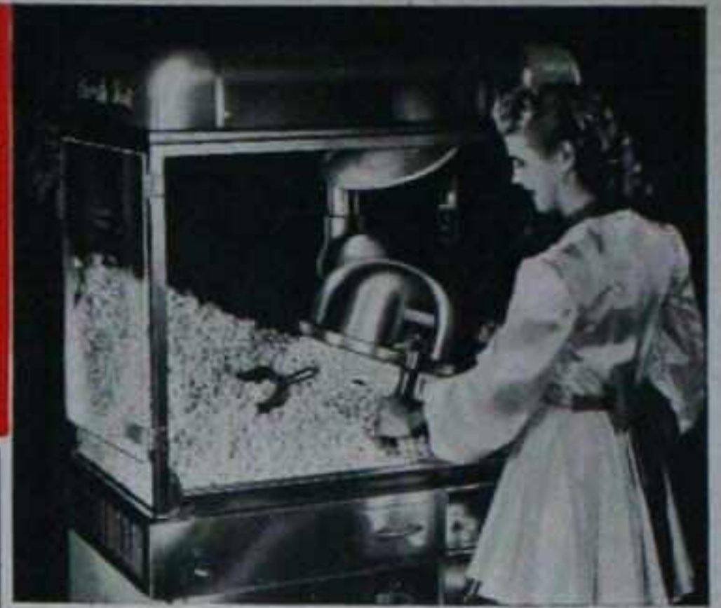
CASCADE KETTLE can be rotated through 360° . . . pressure fingers and collector rings maintain electrical connections as in automobile distributor.
