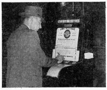
INSUROGRAPH, vending air trip insurance upon insertion of a quarter, is now in operation at Airlines Terminal, 42d Street, New York. After filling in name of beneficiary, flight departure and destination points, signature and other data, customer presses button. Machine then automatically stamps contract duplicates for files, issues original policy to the buyer.
