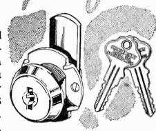
No. 4750 Improved Herculock —pick-resisting design. "Shark tooth" keyway. Double-sided key. Wrench-proof cylinder. key. Wrench-proof cylinder, Extra heavy spur washer, re-taining screws, and key. Cam movement 90 degrees. Thousands of key changes.
