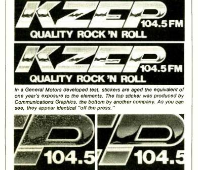
After the test, the equivalent of a year in the weather, note the peeling, fading and cracking in the "label" type product (left). The Communication Graphics decal (right) still looks great
