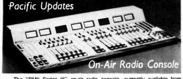
The "BMX Series III" on-air radio console, currently available from Carlsbad, CA-based **Pacific Recorders & Engineering,** features three main stereo mix buses (each with distribution line amplifiers), two telephone mixminus feeds with a monitor mix, and monitor facilities for two separate studios. The unit also sports independent outputs for the console, host, cohost, and guest headphone feeds as well as a stereo cue system with automatic headphone monitor switching.
