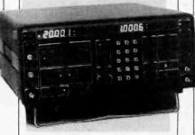
Amber Electro Design has introduced the model 5500, a programmable audio measurement system. It can measure virtually every performance parameter of audio systems and components, including gain, frequency response, output power, weighted and unweighted noise, crosstalk, total harmonic distortion, and intermodulation distortion.
