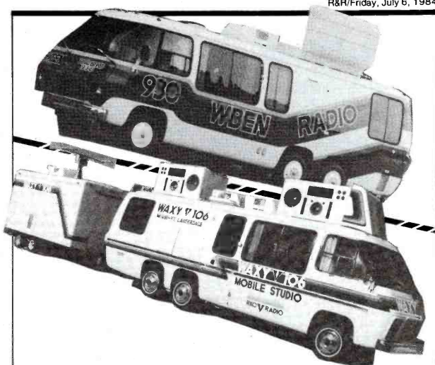
Shown above are WBEN and WAXY remote studios. Both units were built by station personnel from converted mobile homes. The WBEN unit includes fixed and wireless mikes and a production-quality Ward Beck console. Strobe lights are on the roof of the van. The WAXY unit includes a production-quality board plus multiple cart and reel-to-reel tape machines for full studio origination. Located on top of the unit are two television cameras hooked up to monitors inside so the announcer can see all around the truck. Both studios normally send their signal to the main studio via Marti microwave unit.
