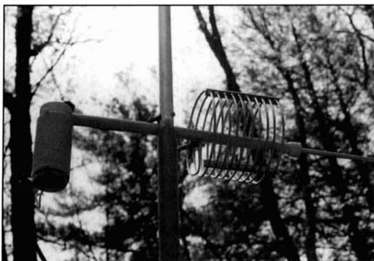
Photo A. Close-up of the 1/2-inch ID PVC cross-arm assembly.
