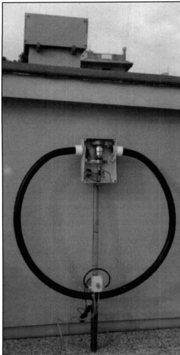
Photo B. The complete antenna showing the connections from the remote tuning to the shack.
