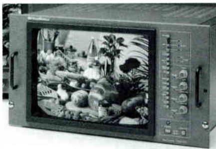
ShibaSoku's CM44A rack-mountable 14" CRT.
