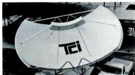
One of ATC's new 70° Simulsat satellite antennas.
