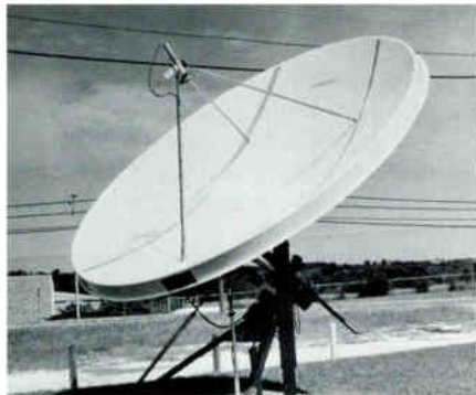
COMTECH's 5.0 meter polar mount satellite receiving antenna.
