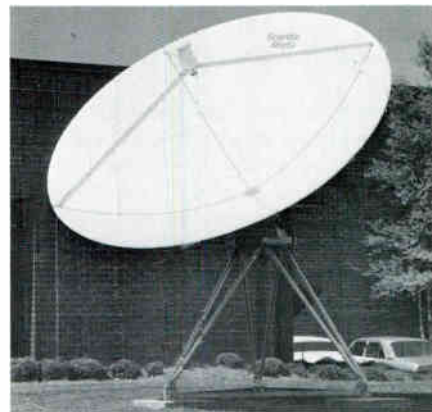
Scientific Atlanta's 4.5 meter receiving antenna.
