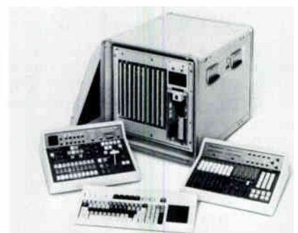
The Grass Valley Group Integrated Production System, IPS-100. The photo shows one of the two optional cases for portability, and the control panels. Note the new JOG-PAD™ at right of edit keyboard.
