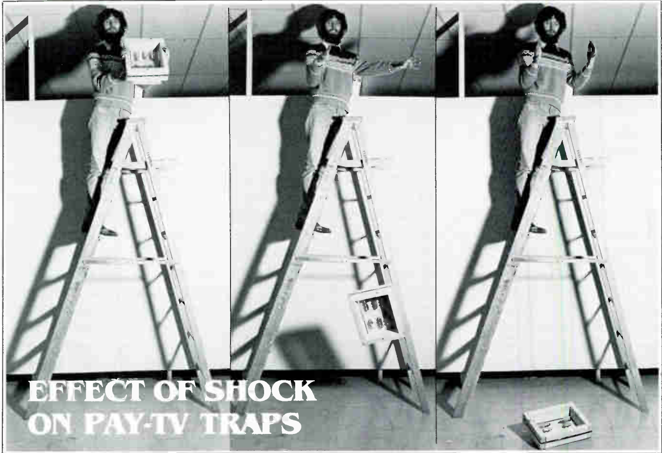
The "SHERMAN SHOCK MACHINE" in Action: Dave SHERMAN drops the trap samples on concrete floor. Samples were mounted in the open wooden fixture, clamped down to prevent connector damage.
