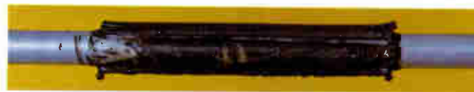
Old Type —Adhesive drips-propagation of pinholes and splits during shrinkage. Not clean stripping.
