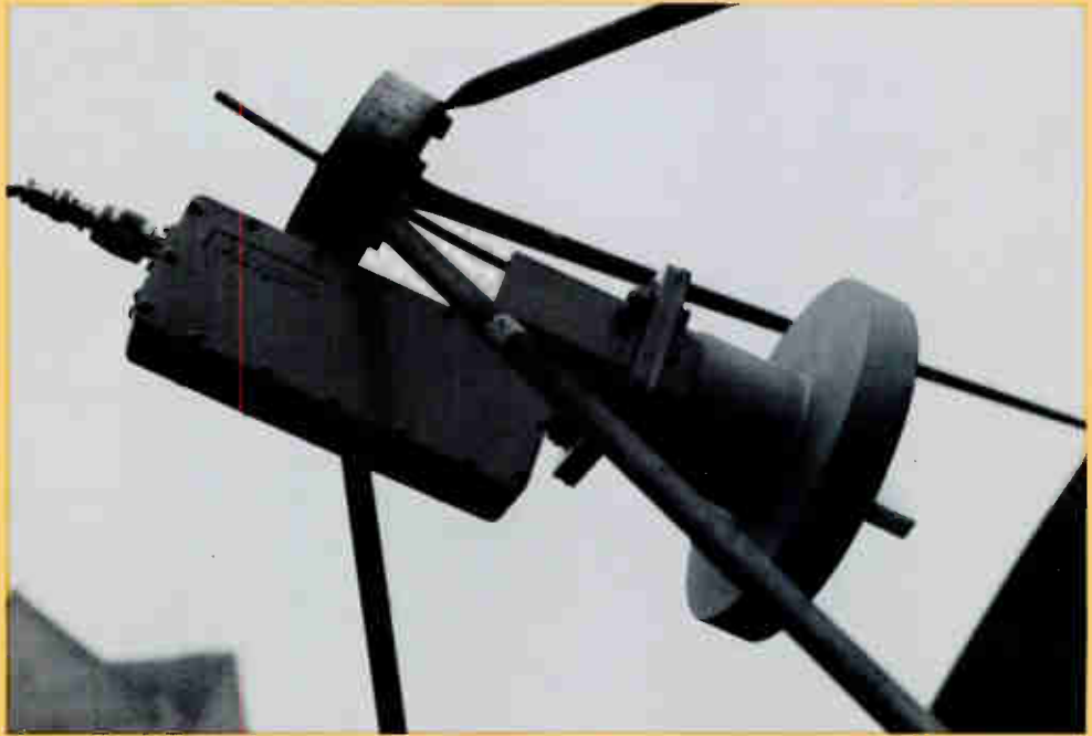
The PTFE Slab Polarizer is just visible in this view of an LNA under test in the author's terminal.
