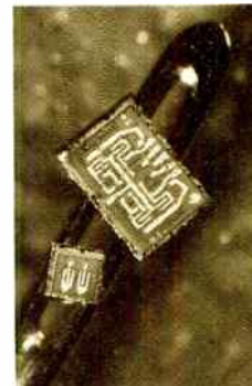
The transistor was invented at Bell Labs in 1947. Today, thousands of transistors can be made on one tiny integrated circuit chip.
