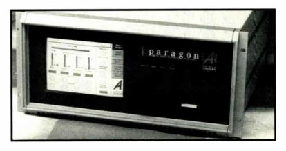
9" VGA touch-screen equipped video monitor; factory-loaded sound library; on-air A/B comparison; remote controllable. *User installable options* will include a Digital 10-band Graphic EQ, Stereo Generator and AES/EBU digital I/O.
