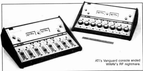
A four-channel stereo console was ordered and installed. The console, manufactured by a prominent US manufacturer, featured FET switching on the input to each mixing channel.
