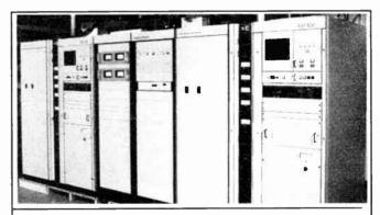
A BE FM-10B M/A, recently delivered to WYNY, includes an optional second center cabinet, Bird RF Wattmeters and a Burk Technology ARC-16 remote control.
