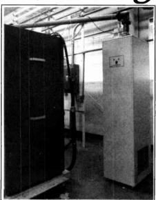
The Altronic Research dummy load, at right, in a typical Continental test installation.
