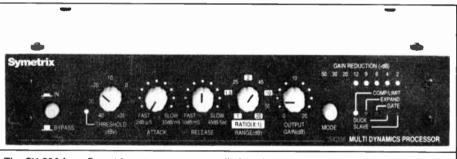
The SX-206 from Symetrix puts a compressor, limiter, downward expander, gate and ducker in a half-rack size unit.
