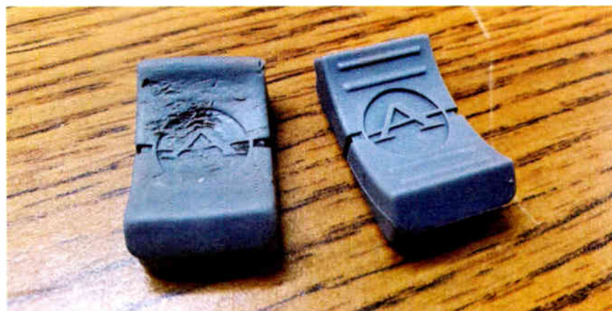
Rubber-coated keycaps can turn to "jelly" after frequent cleaning with non-approved cleaners, such as products with ammonia.
