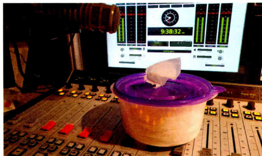
For convenient cleaning, Jim Gray cut a roll of heavy paper towels in three and put them in a disposable Rubbermaid food container with 70% isopropyl alcohol.
