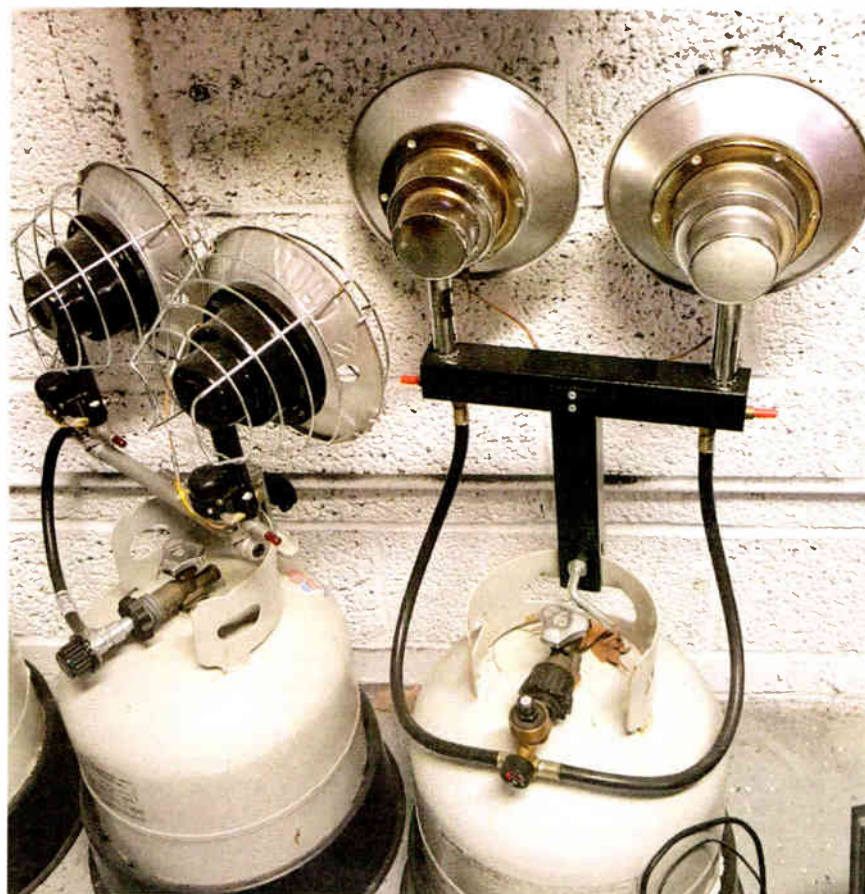
Fig. 1: Portable propane tank-mounted heaters are great for outside work at your tower site come winter.
