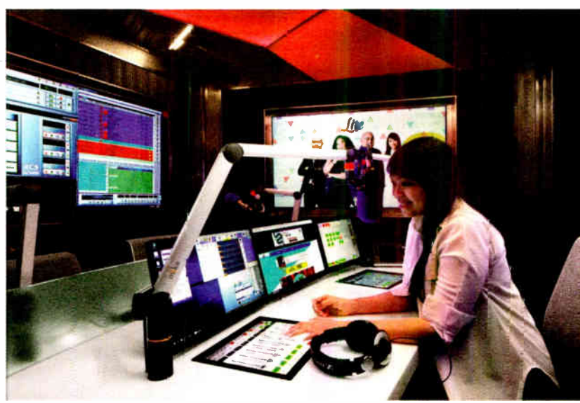
Astro Radio in Kuala Lumpur, Malaysia, uses IP-based radio tools: the control surface is software, driven by a multitouch interface on a high-resolution computer display. LITE channel host Soraya is pictured.
