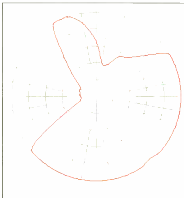
Fig. 1. The author writes, "Pretzel patterns are becoming more and more common in metro areas where FX openings are tight."
