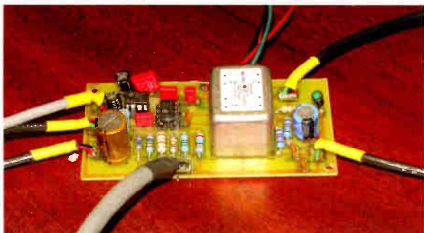
Above: The Version 2 preamp assembly with transformer installed.
