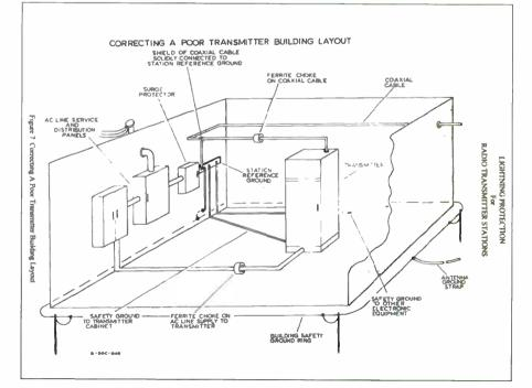
Fig. 3: Reworked ground routing at a transmitter site.
