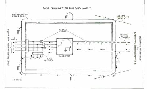
Fig. 1: Incorrect wire routing at a facility.
