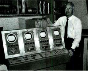
KTLA's chief engineer, John Silva, designed and built the world's first "frame-accurate" videotape editor a decade before the advent of timecode. It used four special Hughes Corp. storage CRT units to freeze a predetermined series of images from the tape, allowing an editor to precisely select in/out-points. It was dubbed on at sign-on, take a set of meter the TV-ola and Silva received a patent for his invention. Silva also pioneered airborne TV reporting with his invention of the "Telecopter."
