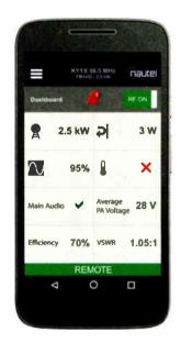
The award-winning Nautel AUI is installed on all modern Nautel transmitters. For all current models, the AUI can be accessed via a web browser. For GV, NV and NX transmitters, the AUI is also presented on a 17-inch front-panel touchscreen. The AUI is designed to give users 100 percent remote access to critical transmitter functions.
