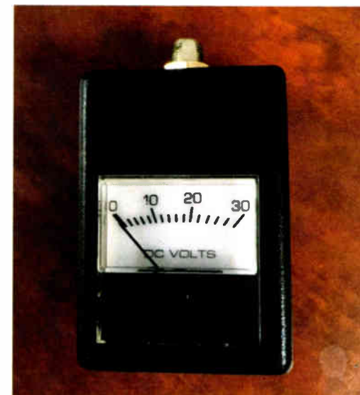
Fig. 4: Tom Weber's LNB voltage measuring device.
