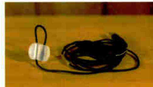
Sennheiser MKE 2 lavalier fits easily inside a Rode Invisilav.
