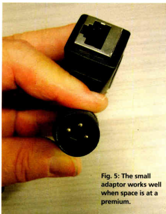
Fig. 4: A compact XLR-to-RJ-45 connector adaptor.
