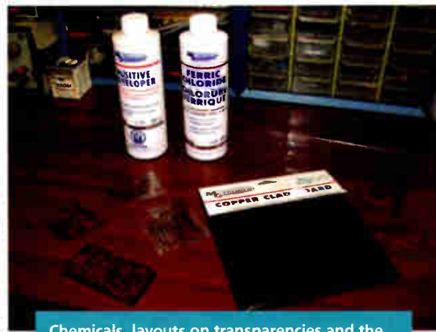
Chemicals, layouts on transparencies and the light-sensitive board are ready to go.
