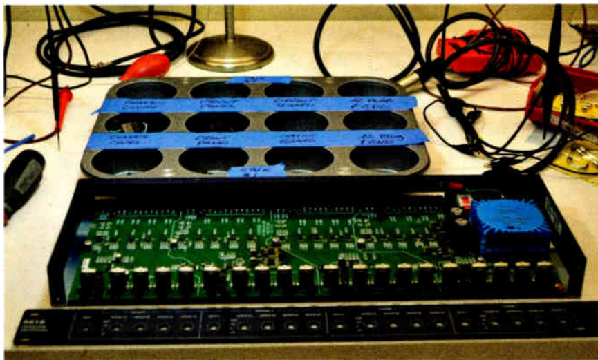
Fig. 2: The DA is ready to reassemble; the muffin tin holds all the nuts and bolts.
