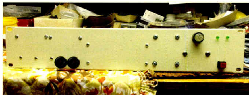
Fig. 4: Two LEDs, in the upper right corner, monitor condition of the regulators.
