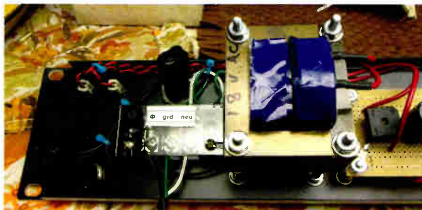
Fig. 2: The power supply section of the amplifier project. Buc used a power transformer from a paging system.
