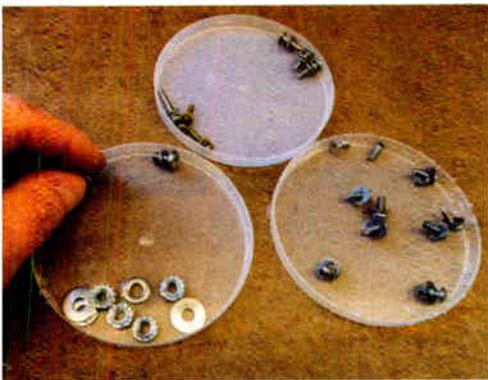
Fig. 3: Plastic boxes from electrical tape make excellent hardware holders.
