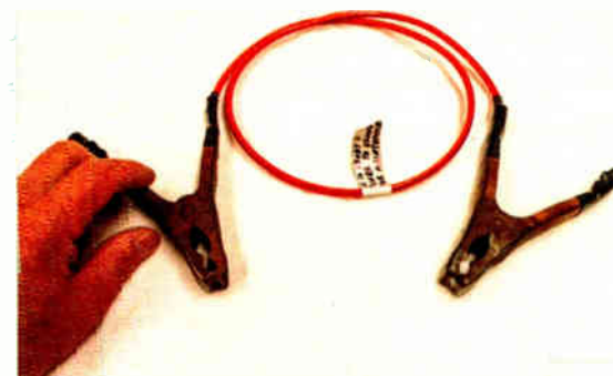
Fig. 4: Cable with alligator clips for shorting an AM tower to ground.
