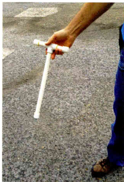
Fig. 1: Made inexpensively out of PVC pipe, this tool facilitates checking buried copper radials.
