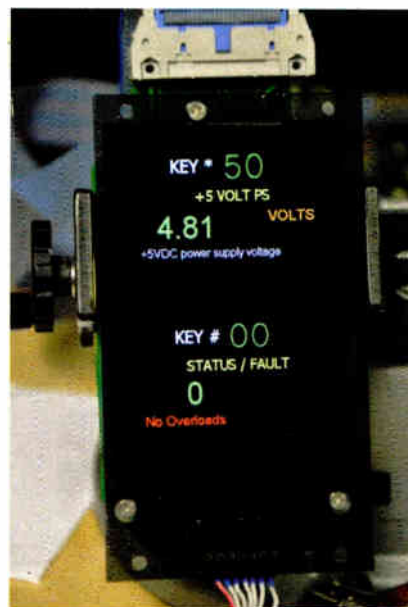
Fig. 2: The MP&A SX Retrofit Display Card solves many of the metering problems of the SX transmitter.
