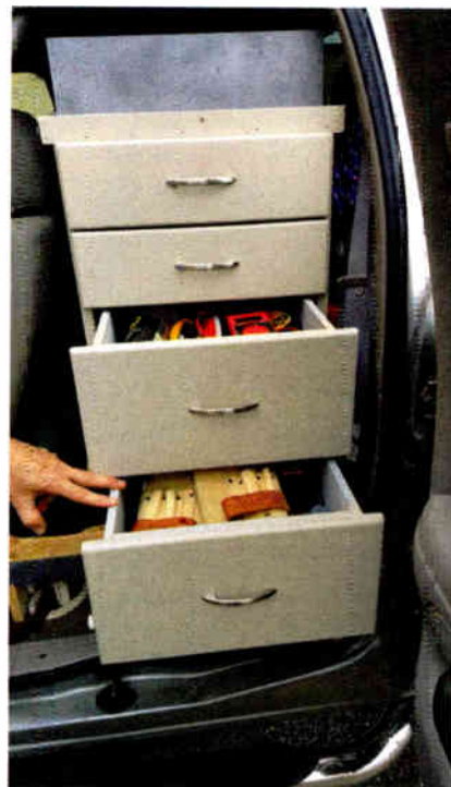
Fig. 1: A multi-drawer cabinet mounted behind the front seat provides storage for the busy broadcast engineer.
