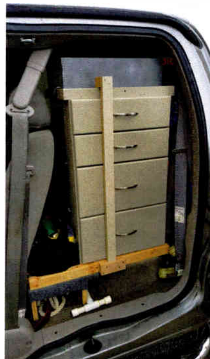
Fig. 2: A wooden slat locks the drawers in place when the vehicle is moving.
