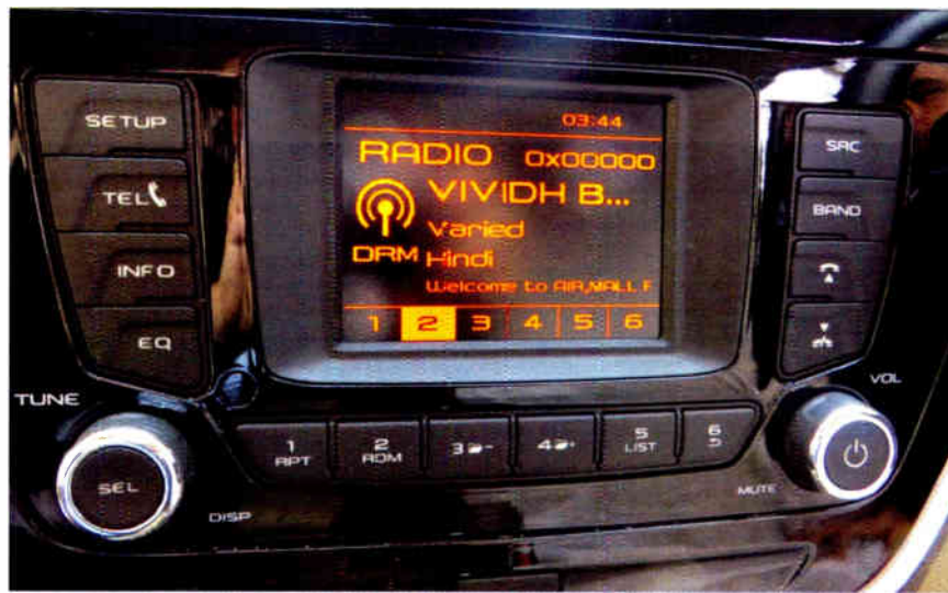
NXP Semiconductors and AIR demonstrated the NXP chip in a DRM-fitted car radio at the BES Expo in February.
