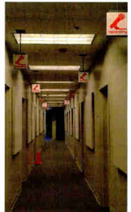
Fig. 3: Suspended on-air lights identify which studio mics are in use.
