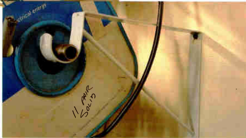
Fig. 2 (below): A close-up of the bracket used to suspend wire reels.
