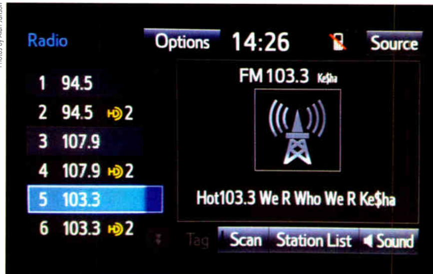
Example of a station transmitting 0xAB to the RDS encoder as recommended in NRSC-G300 to display the U.S. dollar sign ($) in a 2014 Toyota Tundra.
