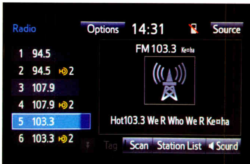
Example of a station transmitting 0x24 ($) to the RDS encoder in a 2014 Toyota Tundra, international currency symbol is displayed instead as per the RDS specifications.
