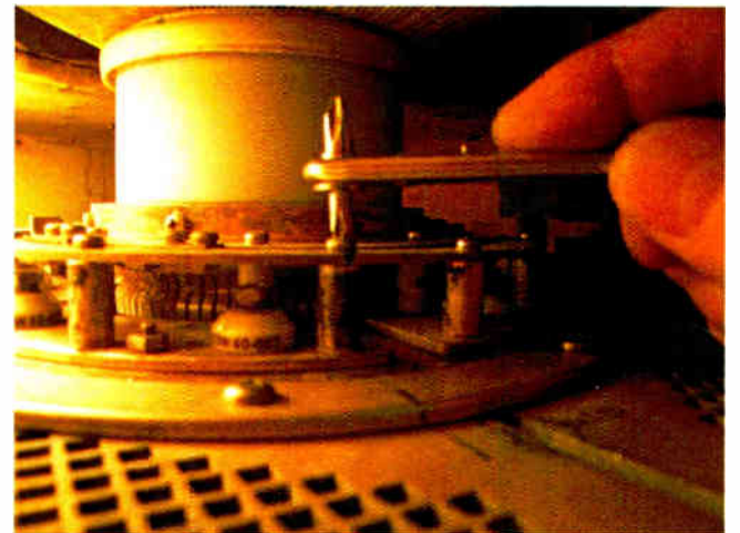
Fig. 8: Installing a screen grid ring in transmitter.
