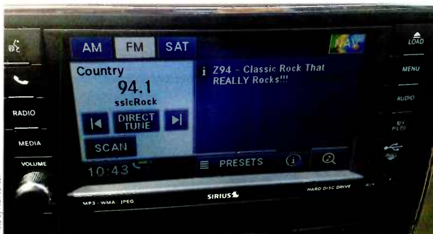
This Classic Rock station is transmitting an incorrect PTY code of 10 for Country instead of 6 for Classic Rock on the author's RDS receiver.
