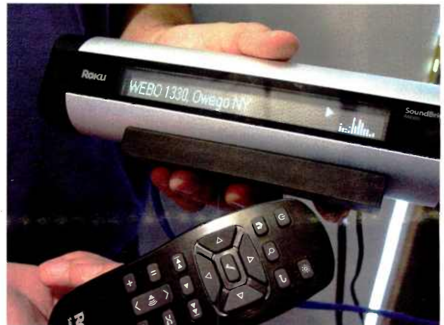
Fig. 2: A streaming receiver provides backup audio should the main STL fail.
