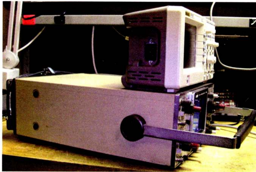
Fig. 1: Side View of Rigol DSO vs. Analog Scope With CRT
