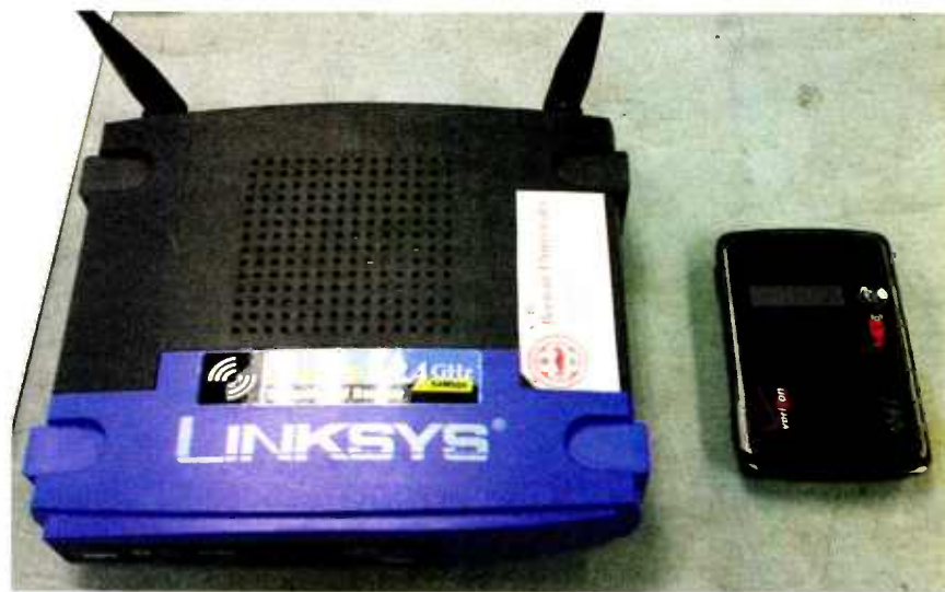
Hacked Linksys WRT54 router and Verizon MiFi. The Linksys receives a signal from the MiFi and connects to the codec via a CAT-5 cable.
