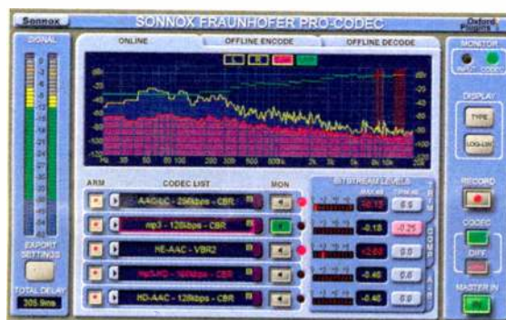
The Sonnox plug-in allows those who are mixing audio to hear what the end product is going to sound like after the MP3 or AAC encoding is applied.
