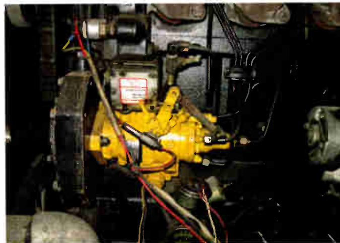
Fig. 2: This one has the fuel-shutoff solenoid replaced with a GAC governor actuator for speed control.
