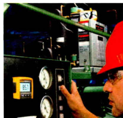
Fig. 2: The Fluke 233 Remote Display Multimeter in action.
