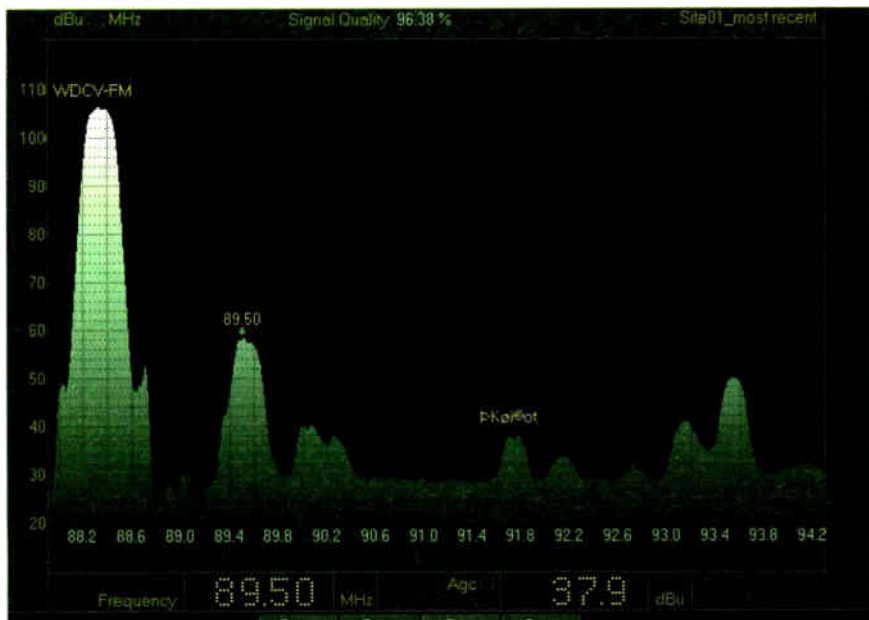
A small segment of the spectrum is shown at 10 kHz resolution. Note garbled information for 91.7.
