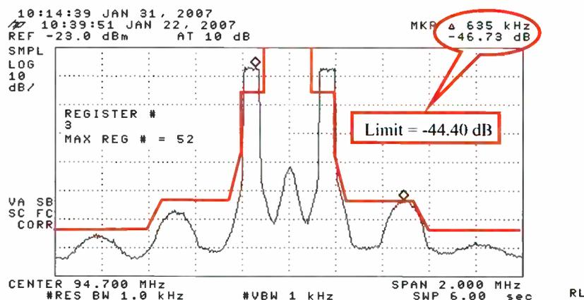
Fig. 2: Typical FM Hybrid IBOC Spectrum @ -10 dB
