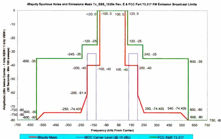
Fig. 1: FM Hybrid IBOC Spectral Test mask @ -10 dBc
