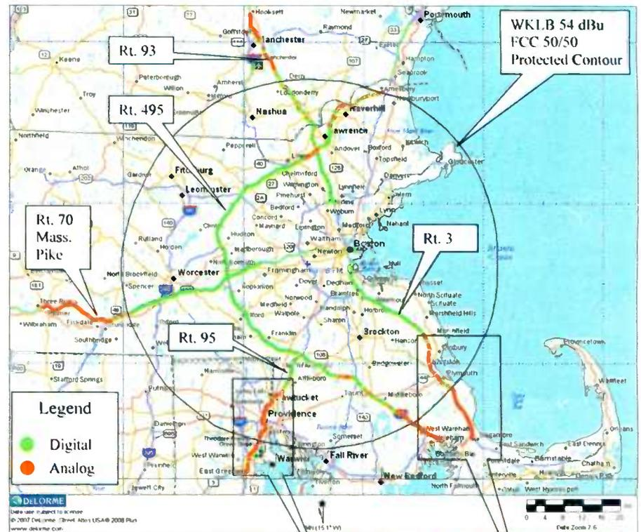
Shown: WKL B @ -20 dBc (-19.21 dBc in Mode MP3). This graphic is referred to as Fig. 5 in the text.
