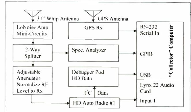
Fig. 4: Mobile Test Platform
