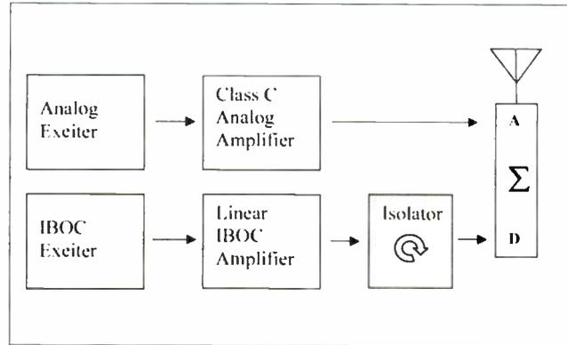
Fig. 3: Dual Input Antenna
