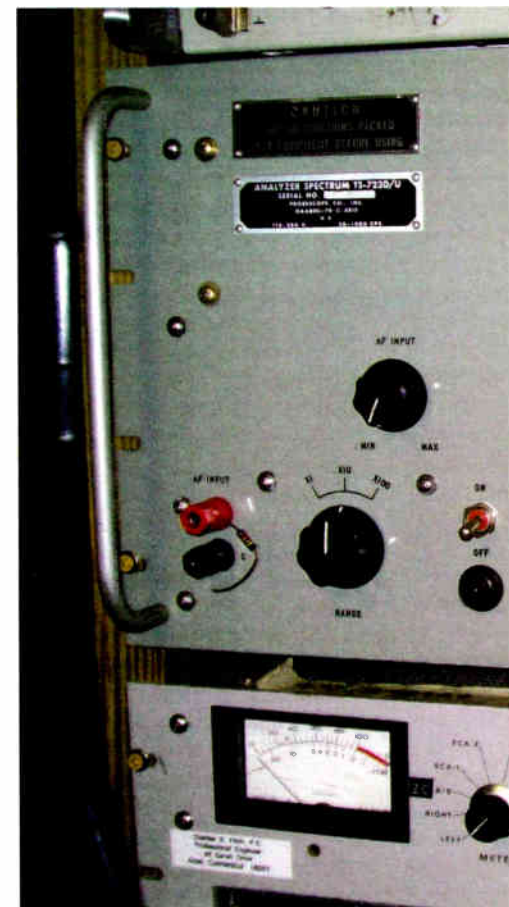
Gone are the days of hauling all that backbreaking test equipment up to the transmitter site such as this classic total harmonic distortion analyzer.
