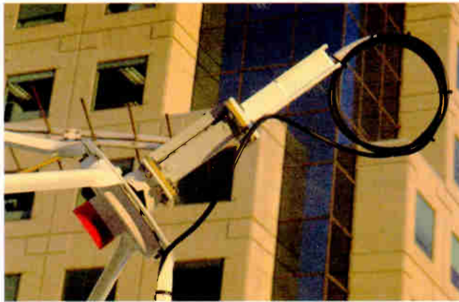
Fig. 1: A radar filter from Microwave Filter of Syracuse reduces interference.
