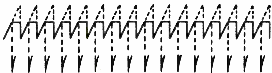
Fig. 1: An extremely linear sawtooth wave was created from the crystal oscillator and applied to the control grid of a triode vacuum tube. With no audio signal applied, the tube is biased to cut off half-way up the slope of the waveform, rapidly dropping the plate voltage and creating a 'spike' through a short RC time constant.
