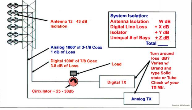
At least one company has been able to achieve greater than -40 dB of isolation between two interleaved antennas.
