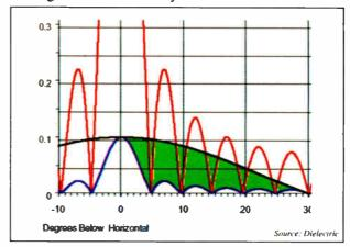
In the hypothetical example in Fig. 1, a two-bay antenna will have one null at a downward angle of roughly 30 degrees from the flat horizon of the antenna, whereas a 12-bay will have 11 nulls
