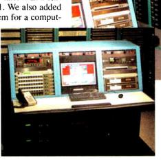
The Frontier console system houses a computer workstation that controls Dial Global's satellite receivers.
