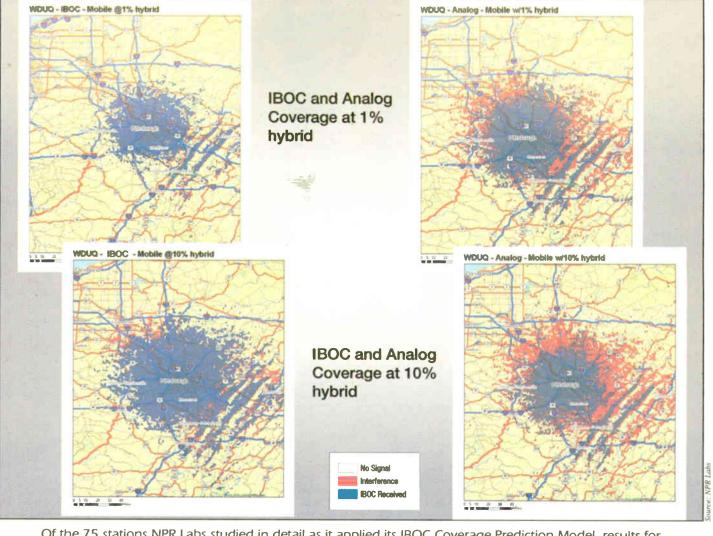
Of the 75 stations NPR Labs studied in detail as it applied its IBOC Coverage Prediction Model, results for WDUQ(FM), Pittsburgh were average in terms of predicted coverage and predicted received interference.
