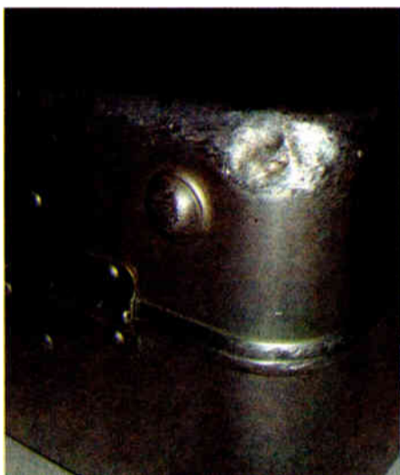
The Zero case sustained only a dent after a 20 foot fall.
