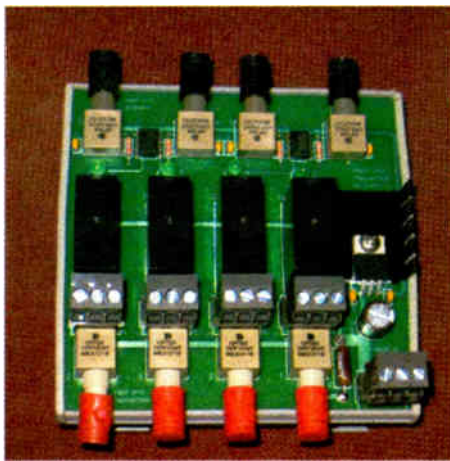
Fig. 3: Fiber-optic loops are terminated in this compact optical module.
