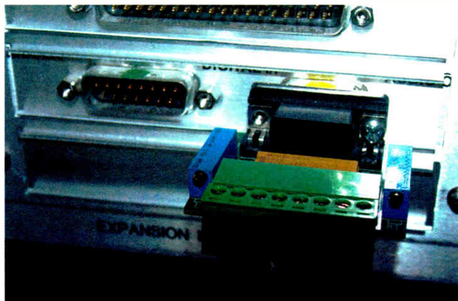
Fig. 2: The Connect O' Pad provides an easy connection for audio and includes trim pots for volume control.
